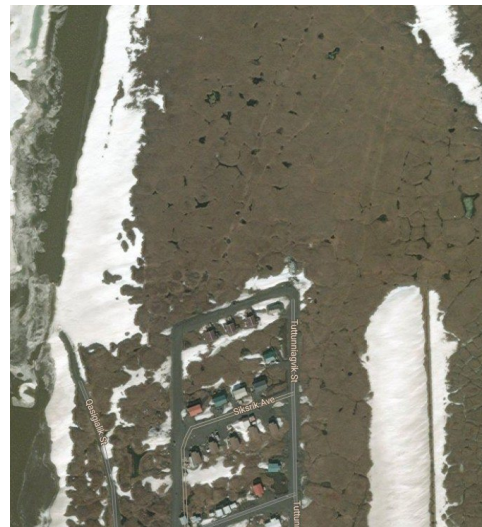
Figure 3: The photography on the left shows a view on the tundra north of Point Lay with clear signs of ice wedge degradation outside of the settlement. The aerial image on the right shows the presence of thermokarst ponds outside of Point Lay (aerial image: bing.com).
