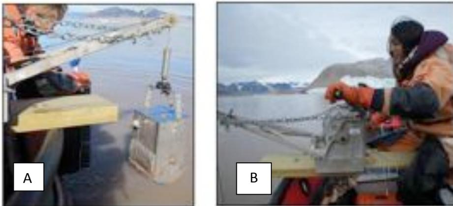
**Figure 5.** Field methods for collecting box core samples. **(A)** Box core suspended from winch over the side of a boat. **(B)** Team member using the winch to haul up a box core.
