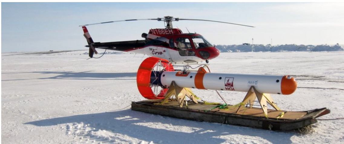
Figure 2.1: MAiSIE: Multi-sensor Airborne Sea Ice Explorer at Roger Wiley Airport in Barrow Alaska. (Photo: Priska Hunkeler)
